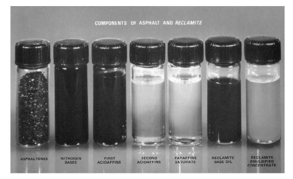
Rejuvenators need to be a fine-particle size cationic, oil in water emulsion of a selected blend of maltene components tailored to facilitate and assure the desired mode of incorporation of the added maltene fractions, into an asphalt pavement. Specific properties are summarized in Table 3.
